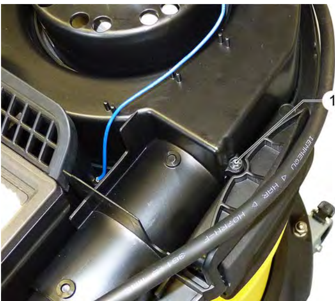
1 Fastening screws, right, suction turbine housing → Loosen the fastening screw.
